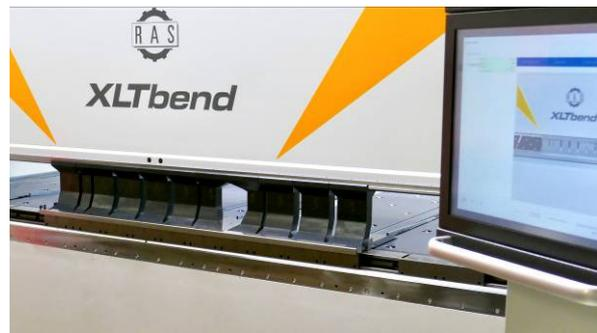
The UpDown folding machine replaced an older bending center. The panel bender was no longer fully utilized, and the XLTbend also offers more diverse bending options for narrow cable trays and shelves.
