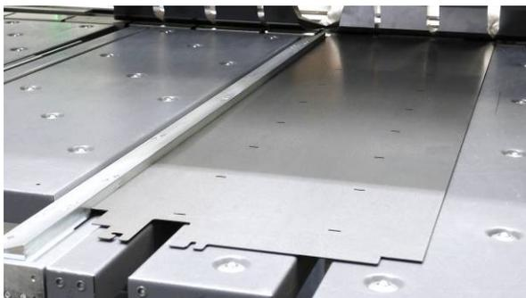
The suction cups in front of the stop units hold the blank to the stop fingers. This means that positive and negative subsequent bends can run automatically one after the other, which is very close to the process at a bending center.
