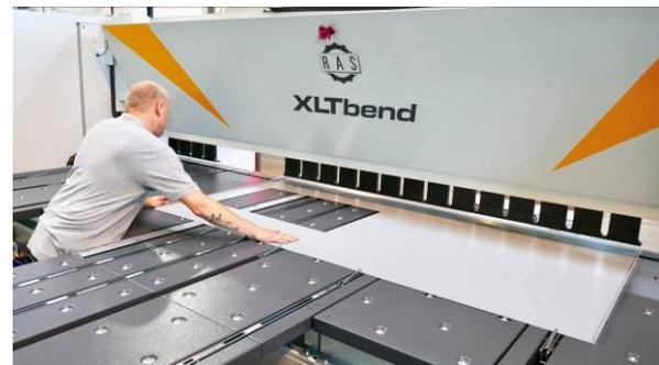
Due to the variety of different sheet dimensions, production batch sizes are small. Head of design Michael Roy explains: "We have stored the most important geometries of our panels in the machine software and usually only change the length and width of these components."
