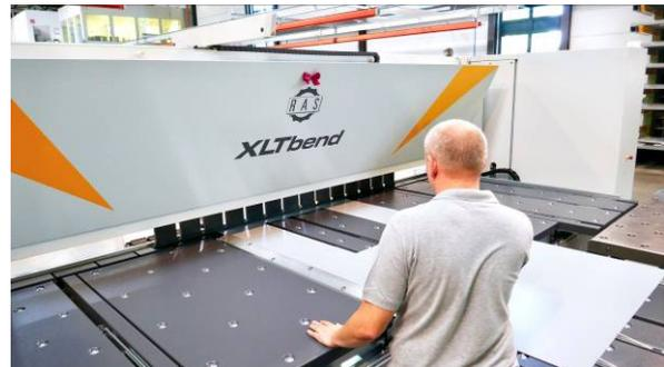
Working from the center of the machine also contributes to the precision of the bent parts. A central stop finger extension increases the standard stop dimensions from 1550 mm to more than 4000 mm. The center working orientation creates an even force curve in the bend, leads to extremely straight bends and reduces the stress on the machine. An additional squaring arm close to the center of the machine simplifies gauging of long and narrow parts.
