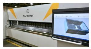
The operator at the machine only calls up the provided program, places the tools in accordance with the setup instructions, and the job can start started. Almost all facade cassettes
