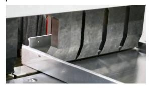
With these automatic sequences, the XLTbend achieves a precision level where the many interlocking components fit perfectly together. Moreover, this quality does not depend on the experience of the machine operator as it would on a press brake.
