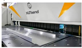
Since many bent parts are visible on the building shell, they must not be scratched during bending - another advantage of the folding technology over press brake bending. The bent parts at BVGlazing are very different in character. Large metal cassettes alternate with slim profiles. The XLTbend masters these special challenges by being operated from the front side of the machine and from the rear. For large cassettes, the worker runs the machine
