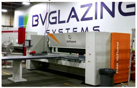
Anyone who imagines a skyscraper with a glass facade probably does not think about how many bent metal parts it contains. The Canadian company BVGlazing has specialized in this industry and bends the parts using a RAS Multibend Center panel bender as well as an XLTbend UpDown folding machine.
