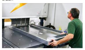
The stop fingers of the XLTbend position the blank for each bend on the bend line. Suction cups in front of the stop fingers hold the part in position. This allows the updown bender to automatically process complete sequences with multiple positive or negative bends without the operator being involved in the actual bending process.
