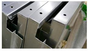
Each architect has different ideas about how the building façade should be designed. Therefore, the number of required components is indeed considerable in tall buildings. As BVGlazing has to deliver the glass modules according to the progress of construction, the total quantity will be divided into several small batches. This requires maximum flexibility and absolute bending repeatability from the XLTbend.
