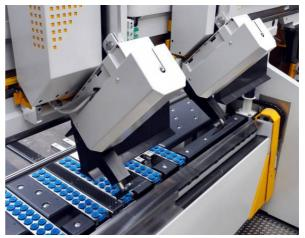
After starting the program, the tool changer sets the upper beam tools automatically in position. Machine operator Fabian Arn says: "The setup of the UpDownCenter is completed in 30-40 seconds. This time I use to load the blank on the machine, align it at the stops and already start preparing the upcoming part."
