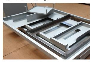
The sound proof enclosures are all individual and built to custom order. The length, width and height change with each cabinet. Sometimes an extraction is needed, sometimes a service door or a window for process control. Markus Augstburger confirmed: "Mostly, each of the about 400 parts of a cabinet is unique."
