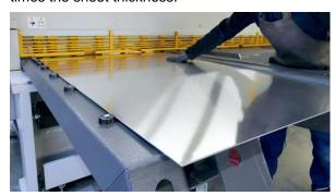
The front area of the shear table is the operator's work area. Its design is essential for easy and efficient handling. Thomas Haag appreciates the ergonomics and says, "The wide, beveled and robust shear tables with embedded ball casters simplify loading and rotating of the metal sheets."
