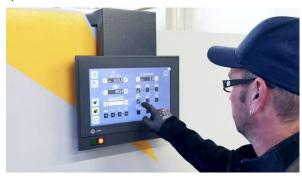
The machine then automatically sets the cutting gap, moves the backstop to position and releases the machine's power for cutting. A sheet support system holds up the blank before cutting and de-
