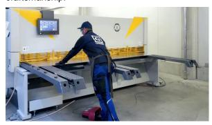
It is therefore not surprising that Gramm was one of the first companies that ordered the new Powercut2 model with a cutting capacity of 6.3 mm and a working length of 3190 mm. Gramm has chosen the extended 1500 mm sheet support
