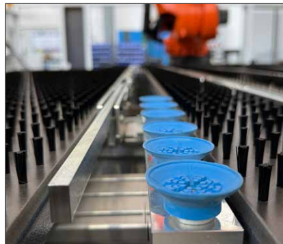
3-in-1 hybrid backgauge with increased suction power and an independent vacuum pump
