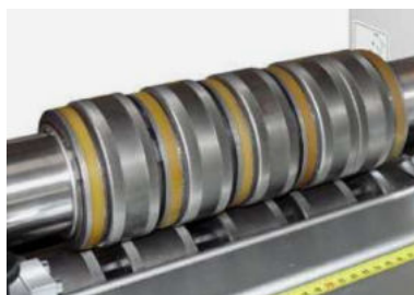
Rolls for standing seam and snap-lock seam.
