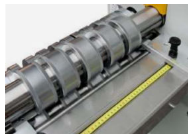
Tape measure for quick roll positioning.
