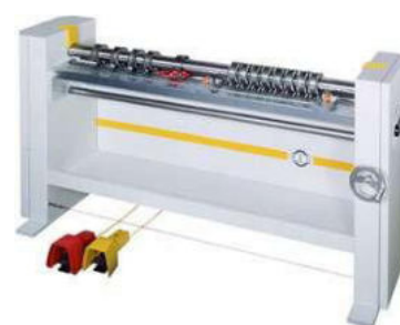
Foot switch for variable speed and rotation direction.
