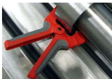
Stiffening pliers reduce shaft deflection for consistent radii.
