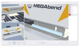
${\sf A}$  3D simulation shows the bending sequence, the tool setup and the loading position of the part.
