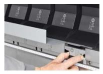
With the DownTools, inward offset bends can be produced without an additional tool setup.
