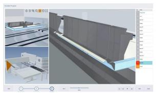
The bending programs can be created with offline programming software in the office without blocking the runtime of the machine. The Bendex software programs the bending sequences automatically. Salzmann's bending team uses the geo data of the part geometries as a starting point.
