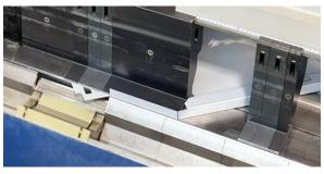
Small flanges from the neighboring part sides protrude above the bending line and may not be bent. This is where the RAS panel bender uses the UpDownTools. They automatically fold in on themselves and thus allow segmented bending operations.
