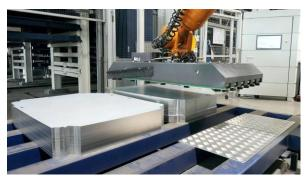
For bending panels and cassettes up to 2560 mm bending length and up to 2 mm mild steel, 3 mm aluminum or 1.5 mm stainless steel Salzmann
